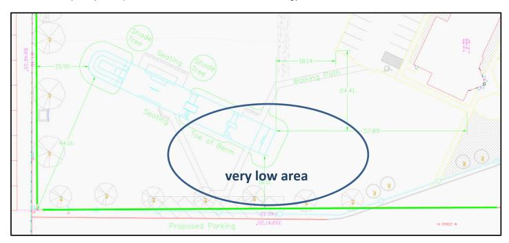
Revised site plan (been shifted to be visible, but avoid the very low area to reduce the fill required):
