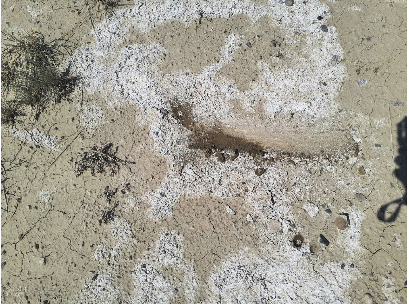
Photo 5 View of the distressed vegetation, white crust, and results of the surface scrape test showing the soil beneath, in the northern section of the Site
